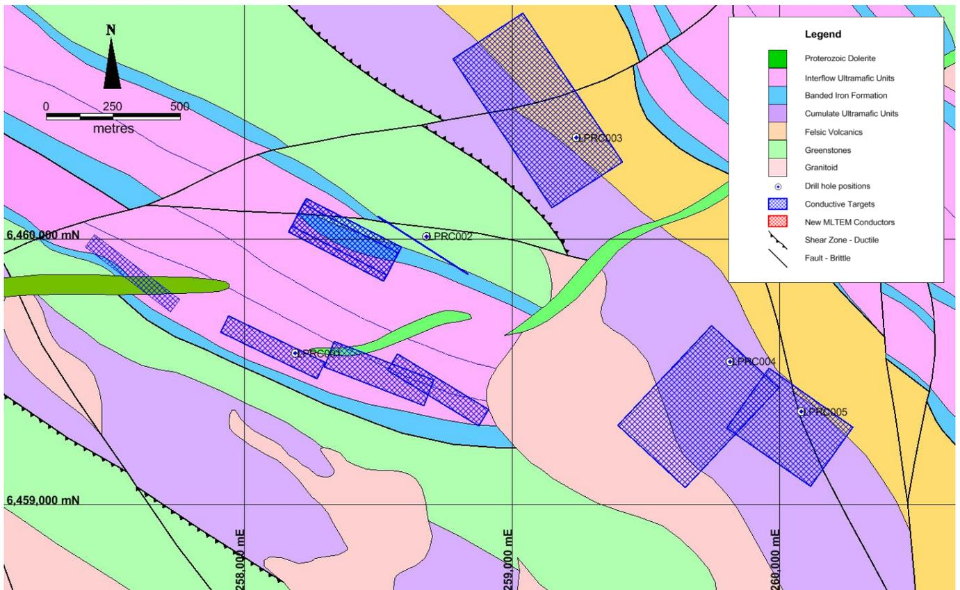
**Figure 3** Lake Percy geological interpretation showing drill hole positions and conductors along the contact between the ultramafic and sedimentary units. The geology is dips steeply to the west and the conductive plates shown are between 100 and 300 metres below surface
