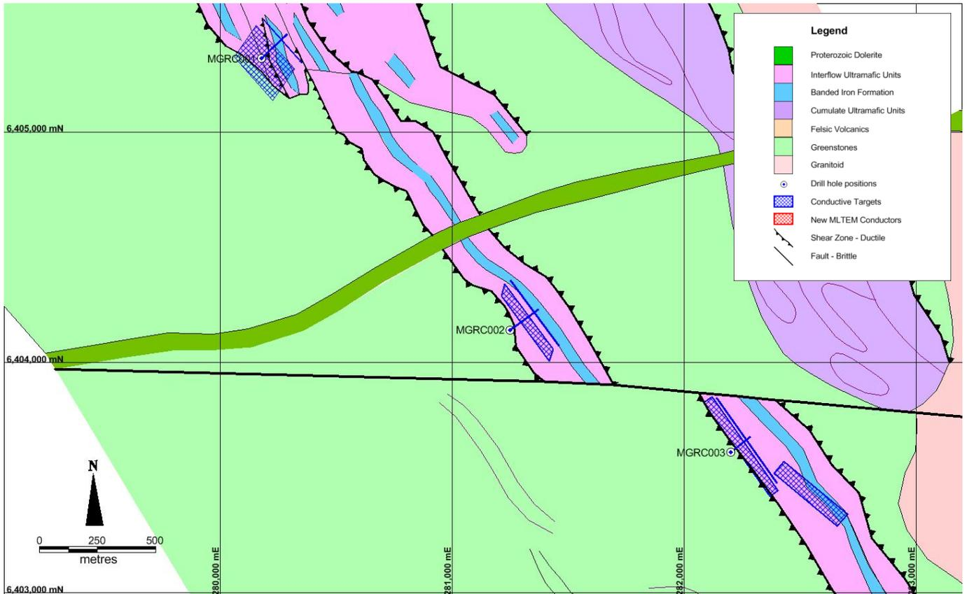
**Figure 2** Mount Gordon geological interpretation showing drill hole positions and conductors along the contact between the ultramafic and sedimentary units. The geology dips to the west and the conductive plates shown are between 100 and 300 metres below surface
