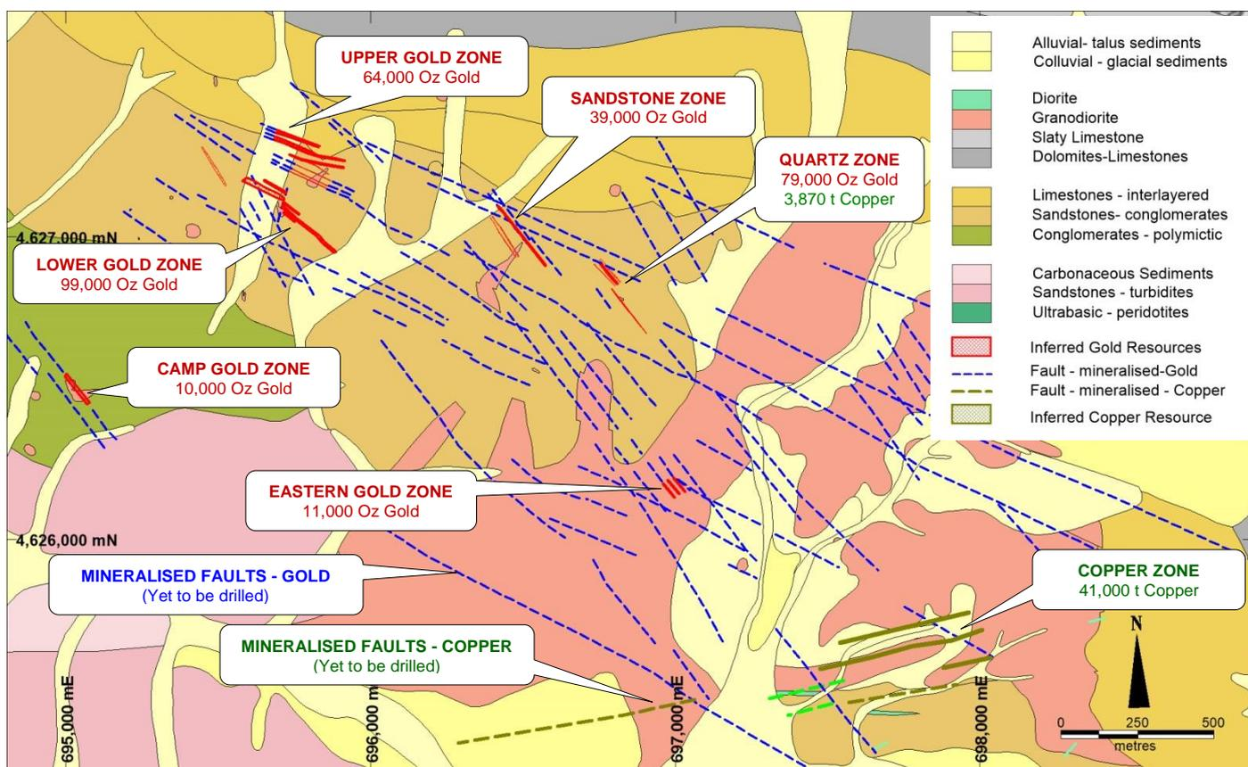
**Figure 1:** Location map of drilling showing Inferred gold resources (red hatch) that represent less than 5% of the identified mineralised faults. 95% of the mineralised faults identified by rock chip sampling are still to be drilled (dashed blue and green lines)
