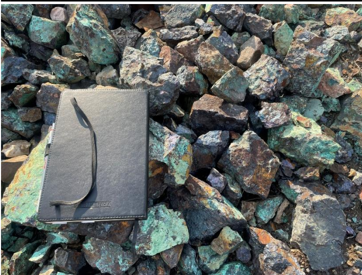
Figure 14: Copper mineralisation (oxide and sulphides) at Bornite Lake
