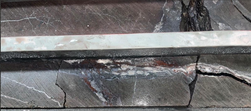
Figure - Photograph of cut NQ2 diameter core containing vein-hosted chalcoite from 66.4m downhole in DAN26026
