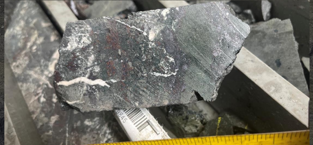
Figure - Photograph of halved NQ2 diameter core showing mixed chalcoite and bornite mineralisation in the chlorite breccia zone at 45.5m in DAN26026
